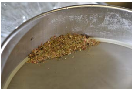
Step 7 to 11: Organic matter is weighed and half is grinded for DNA extraction.
