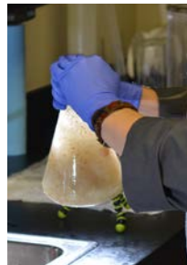
Steps 3 to 6: Organic matter is removed from original sample through decantation.
