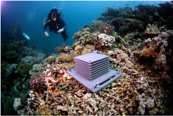
ARMS deployed in Indonesia, anchored using 4 stainless steel stakes
